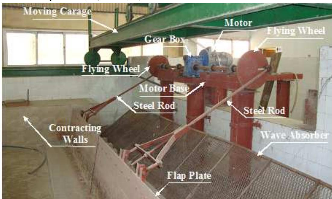
**Photo (13) Different components of the wave generator**
