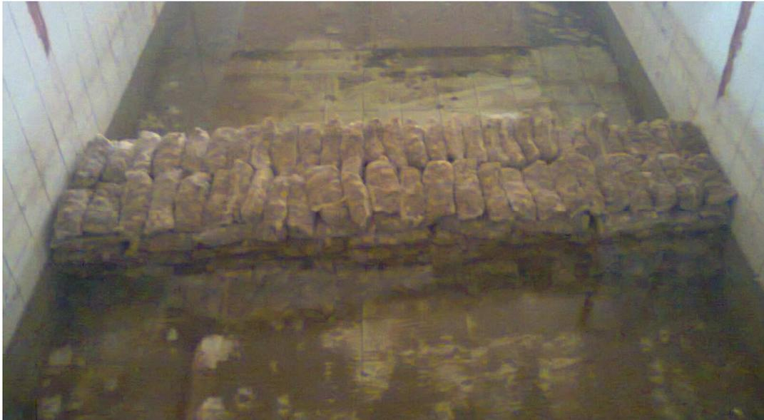
**Gabions Filled With Rubble Used As Submerged Breakwater**
