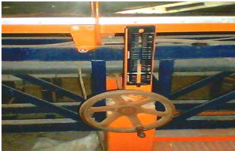
**Photo (18): Changing flume bed slope part**
