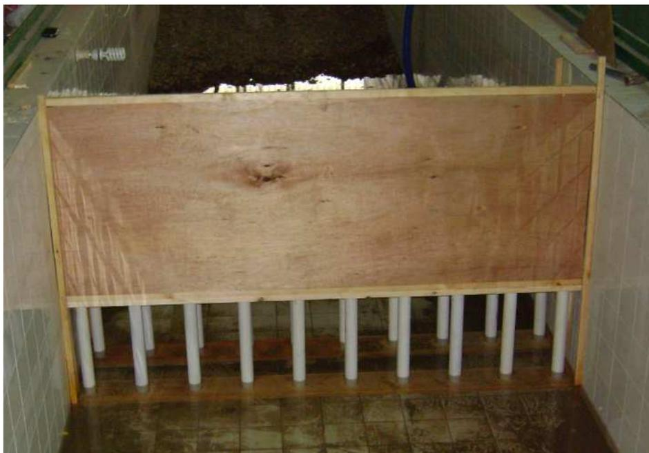
**Vertical suspended breakwater supported on piles**
