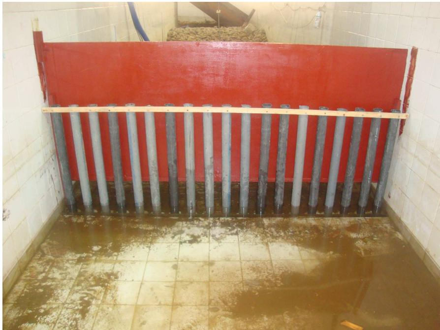
**Caisson breakwater supported by two rows of piles**
