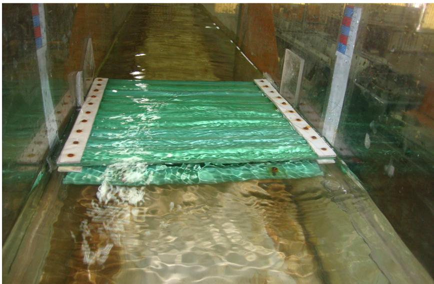
**Horizontal half pipes breakwater model.**
