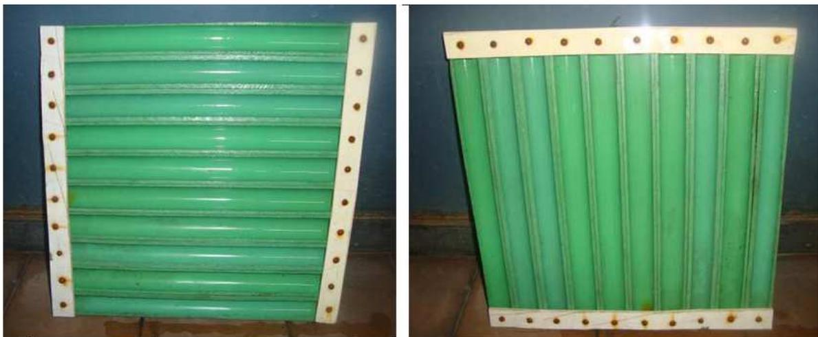
**Vertical half pipes breakwater model.**
