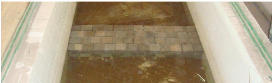
**Vertical submerged breakwater model**
