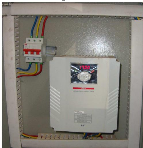
**Photo (14) Wave generator control unit (Inverter circuit)**
