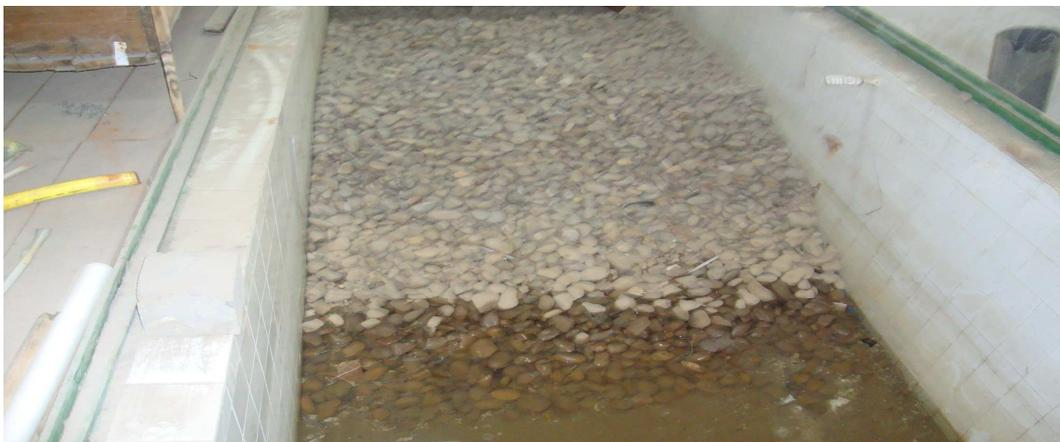
**Photo (7) General view of the end wave absorber**
